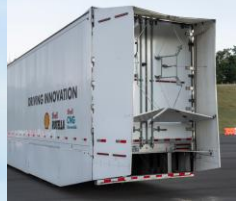
Boat tail streamlines air flow to reduce drag
