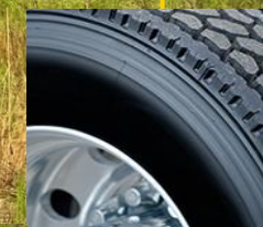
Bridgestone wide-based, low-rolling resistance fuel economy tyres on the truck and trailer
